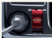
Distress button with a spring-loaded cover
